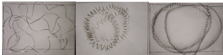
Figure 8: Chips formed under NTMPE
