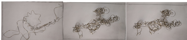
Figure 7: Chips formed under dry Machining
