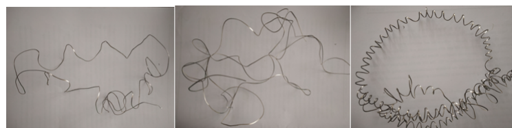
Figure 9: Chips formed under Conventional mineral oil
